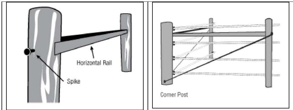
If your corner, end or gate post is large in diameter, you may want to pre-drill a hole for the spike through the post and into the end of the rail.
