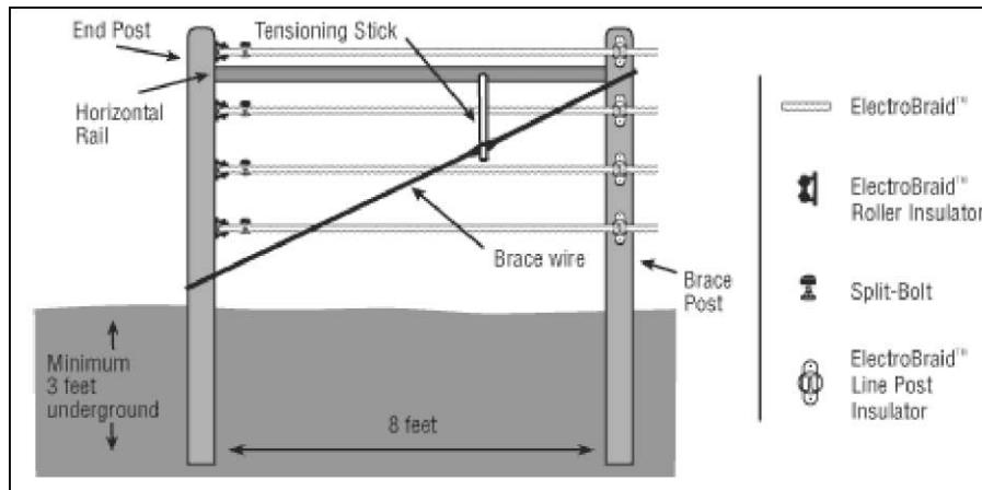
Whenever you fence a long, straight run you need to terminate and install a brace system every 2400 feet to maintain tension on the Braid™.
