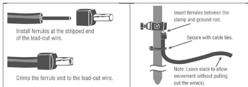
Secure connecting wires to the ground rods with brass ground rod clamps. Add cable ties for increased security. After all ground rods are connected, connect one ground rod to the negative terminal on your energizer.
