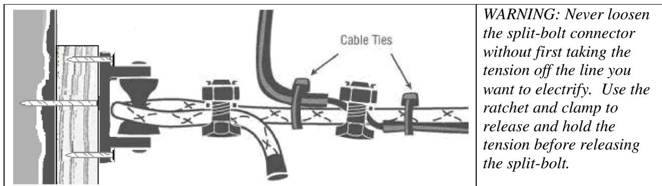
*NOTE: For easier troubleshooting, it is best to use an extra Split Bolt Connector to connect your electrical components. If you want to disconnect the electrical from a strand you will not have to use the tensioning device to hold the tension.*
