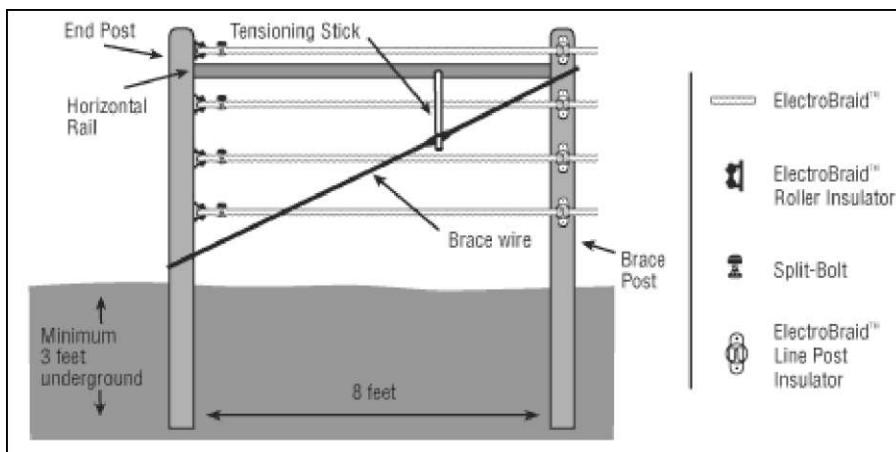
*NOTE: To prevent an electrical short, make sure the brace wire and tensioning stick cannot contact any ElectroBraid™ strands*
